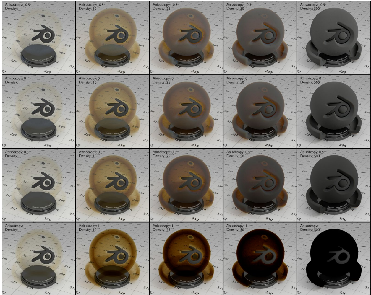
Fig. 2.23) Renderings with a volume scatter material. From left to right the density was increased, the values were: 1, 10, 25, 50, 500. From top to down the anisotropy was set to -1, -0.5, 0, 0.5 and 1. Notice that a volume scatter material with a high density looks fairly similar to the diffuse shader. The color of the shader is the same powder blue I use for all of the test renderings, the appearing color however is its complementary color, since blue got scattered away. The grey parts are where the scattered powder blue mixes with it's complementary color, which is most visible for high densities.
